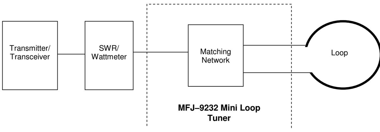
**Figure 3: Typical MFJ-9232 *Mini Loop Tuner*™ Configuration**
